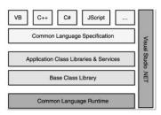
The diagram shows the various functionalities of the .NET framework. The other components such as the Visual Studio Net are also shown here. The base of the functionality of the program is the operation system. The other components comprise of the application class libraries and CLR. This the structure that makes the complete architecture very robust and user friendly.
